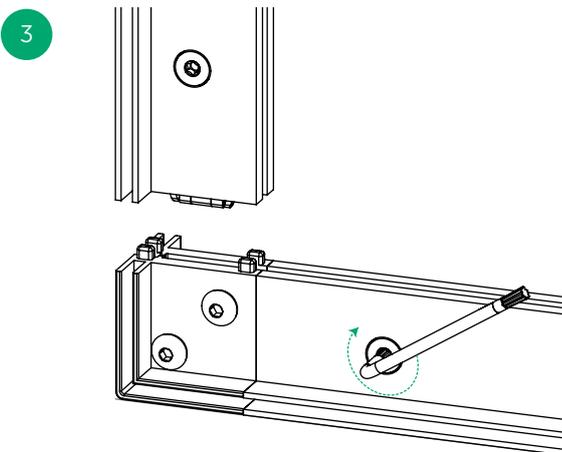
3 | Once the knuckle is in place, tighten each lock using a lock key to secure the corner.
