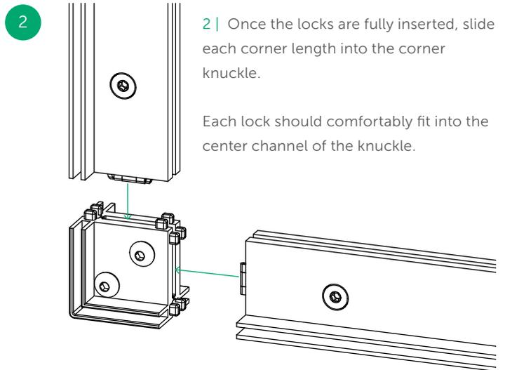
2 | Once the locks are fully inserted, slide each corner length into the corner knuckle.
