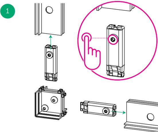
1 | Begin by inserting the locks into the corners by simultaneously pushing down the lock button and inserting into the channel.
